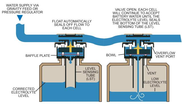
AIR PRESSURE IN THE (LST) STOPS WATER FLOW INTO THE CELL WITHOUT ANY MOVING PARTS.
